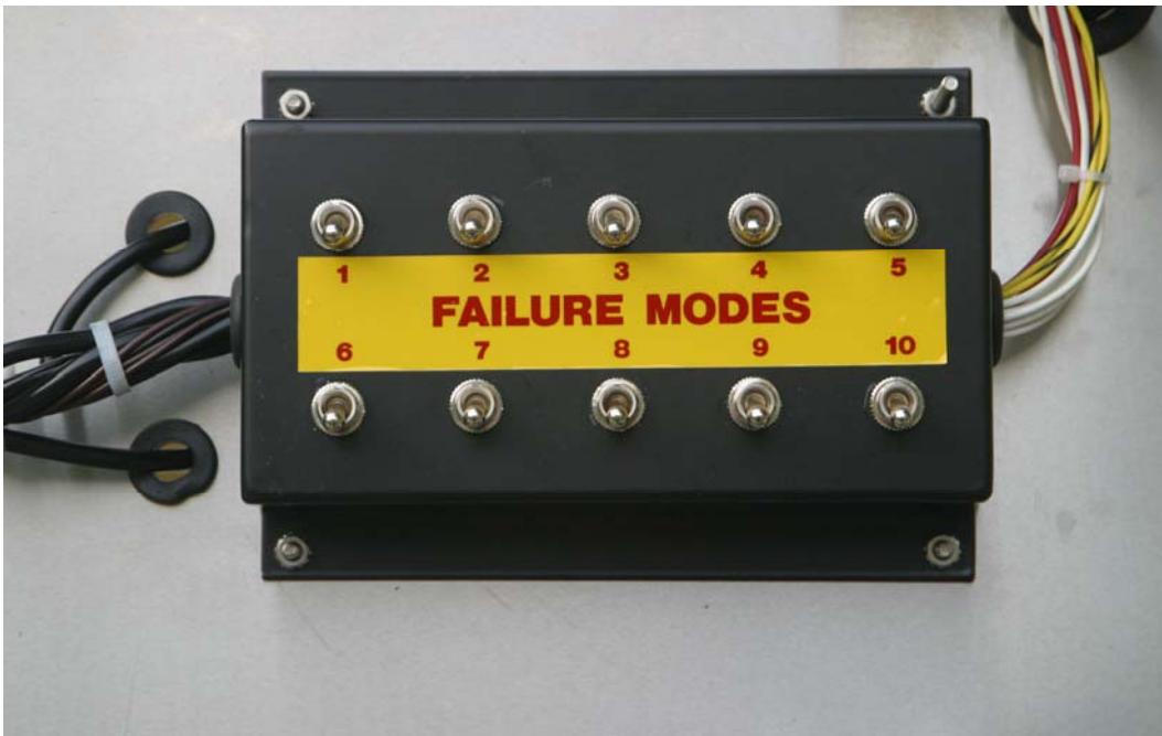
Close up of the Failure Mode Panel (28)
